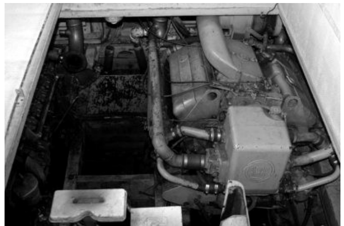
POWERED BY GM DETROIT 8V-53 ENGINES WITH TWIN DISC MG 506 GEARS
