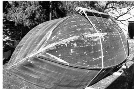
BOAT ROLLED WITH PULLEYS AND FRAMES
