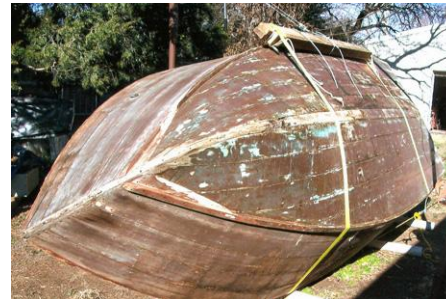
BOAT ROLLED WITH PULLEYS AND FRAMES
